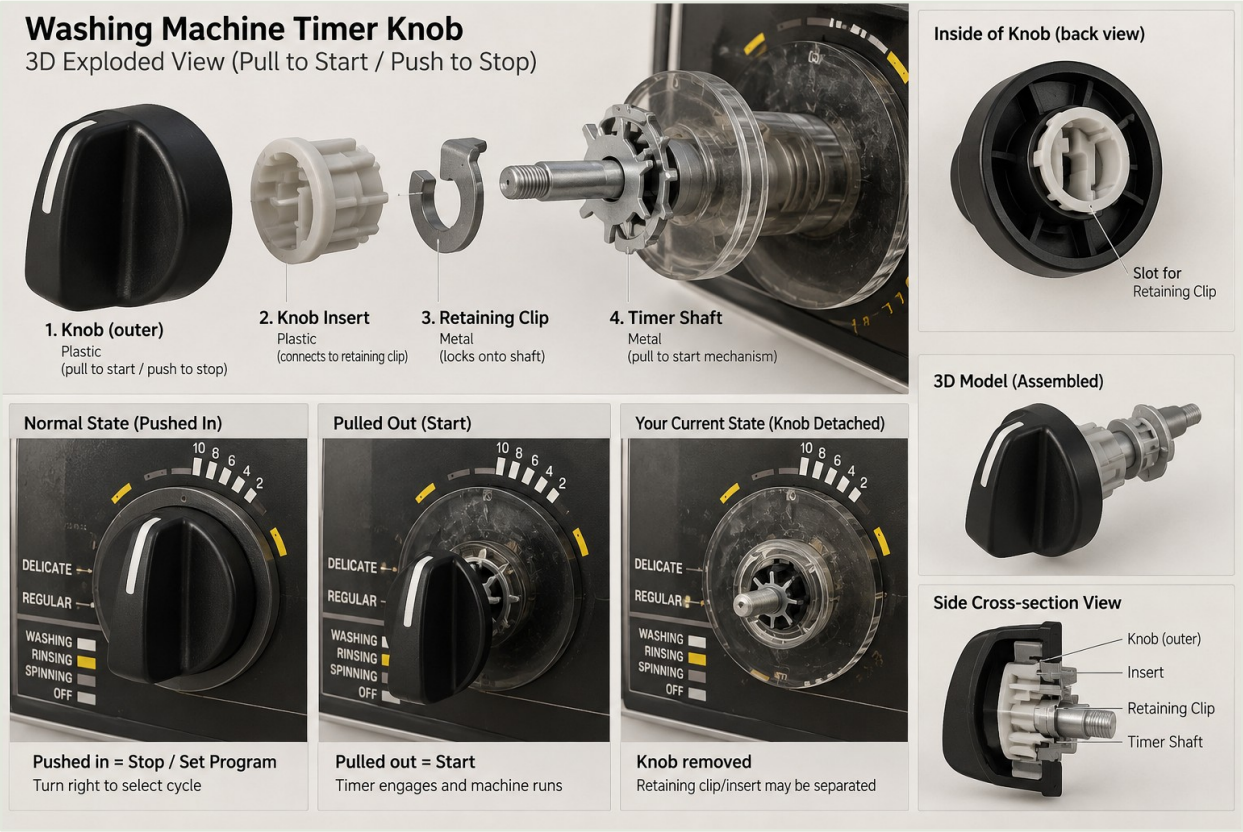
Timer knob — outer knob, insert, retaining clip, timer shaft.
